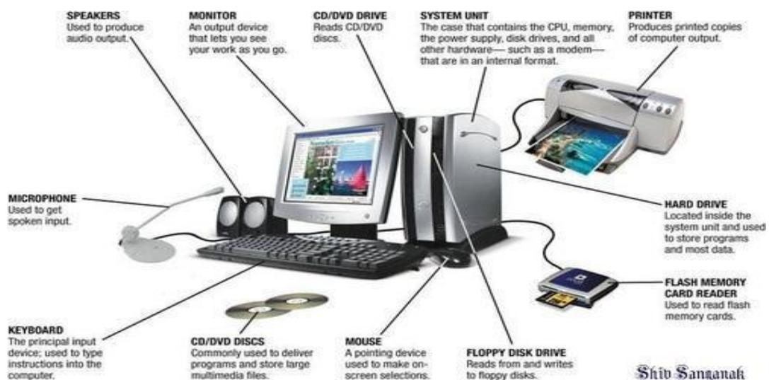
Fig 5.3.1: Components of a computer
