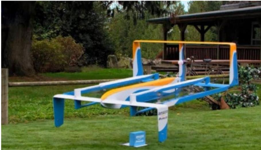
Figure 4.1. 4 Hybrid drone
